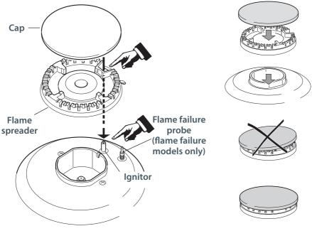
Fig. 18 Correct line-up of auxiliary, rapid and semi-rapid burner parts
